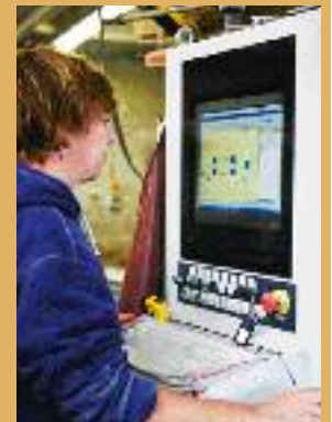
This new, state-of-the-art Computer Numerical Control system can be programmed with a template which then cuts the stone automatically
